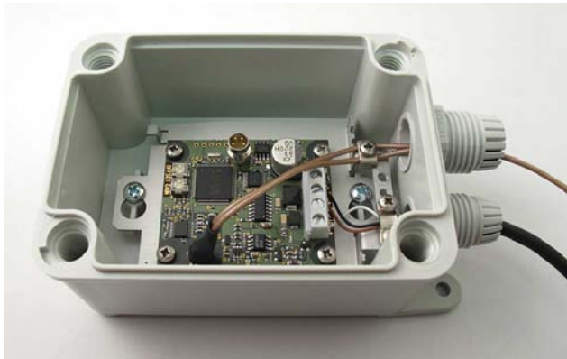
Figure 5 Bracket Installed and Cables Connected
