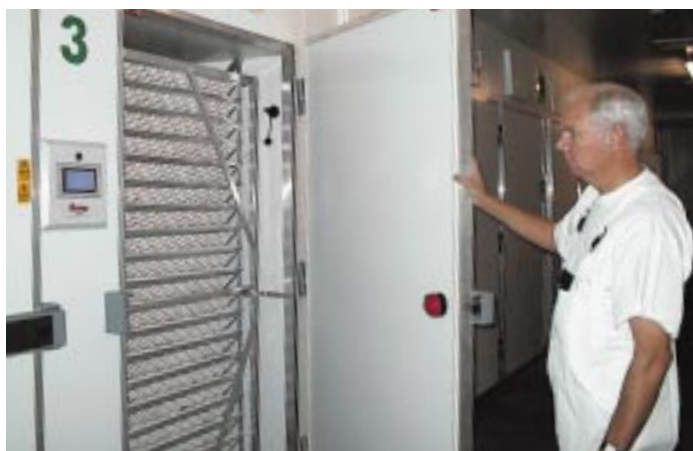
Brian Hodgett, Buckeye's Technical Consultant inspects the trolley turning system.
