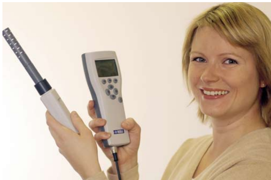
The MI70 connected to a GM70 diffusion sampling probe measures CO 2 concentration. It is a handy tool for spot-checking measurement.
