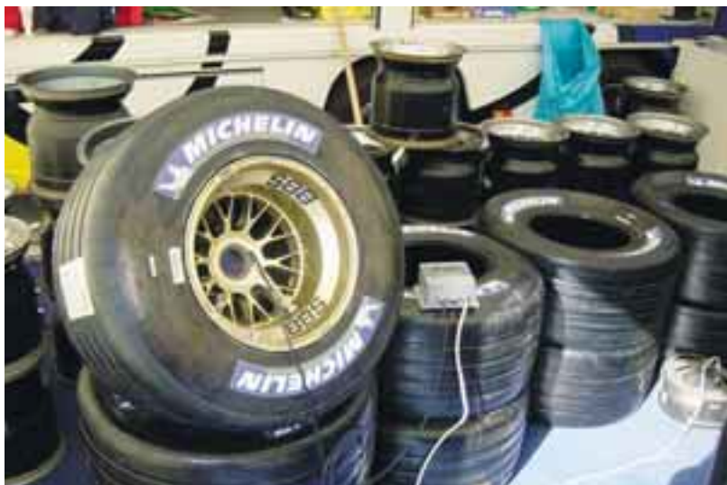
Much of the performance and speed of F1 cars depends on the tires. For different weather conditions, Michelin produces three different types of F1 tires: dry, intermediate and wet. A Vaisala HMP238 transmitter measuring humidity in tires.
