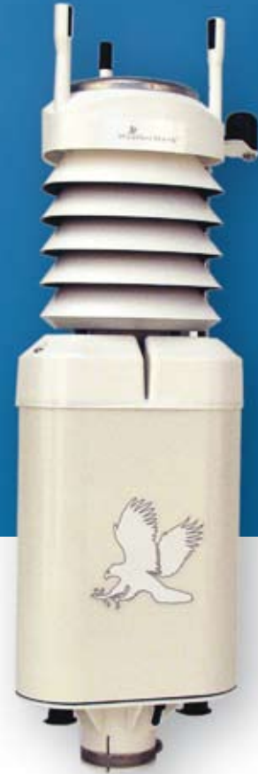
WeatherHawk Series 500 Weather Station with the Vaisala Weather Transmitter WXT510.
